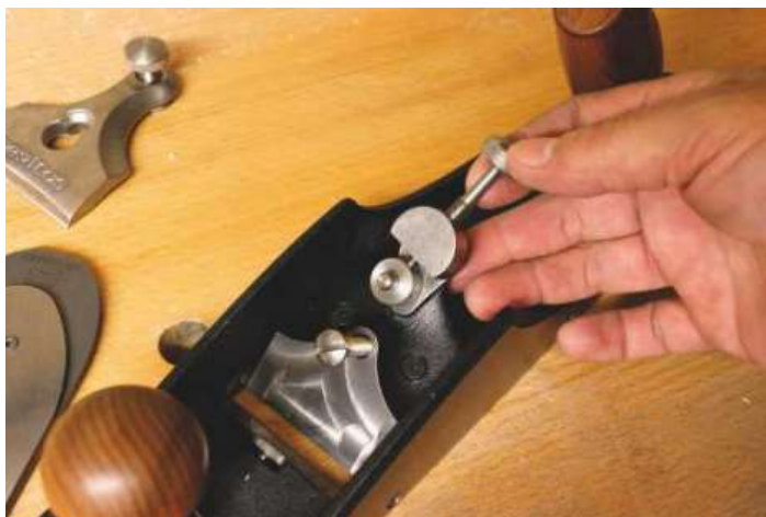
▲ The Norris-style adjuster is beautifully engineered and works flawlessly
